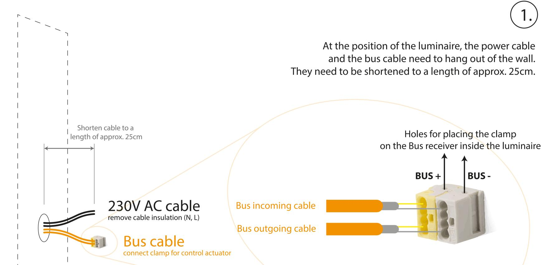
Clamp for Bus cable Choose one pair of cable cores for the BUS+ and BUS- signal.
